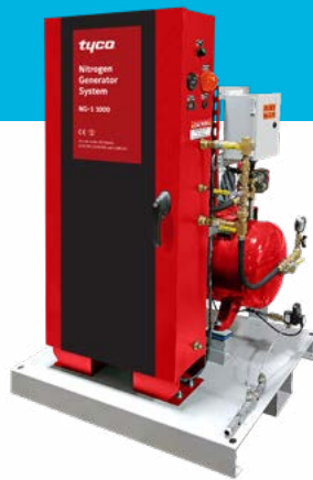
Skid-Mount Nitrogen Generators FM Approved, CE Certification, UL 508A Listed control panel, integrated oil-less air compressor with air receiver tank. Available in the Americas only.
