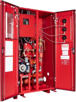
Valve Cabinets The Red-E Cabinet is a pre-assembled, pre-wired and pre-tested fire protection valve package designed to occupy minimal floor space and provide an enclosure for the valve riser. The valve riser has a grooved connection to minimise installation time. Unit also features industrial-grade rollers for mobility and is forklift-compatible. Customised cabinets with the required options are available for tunnel applications.
